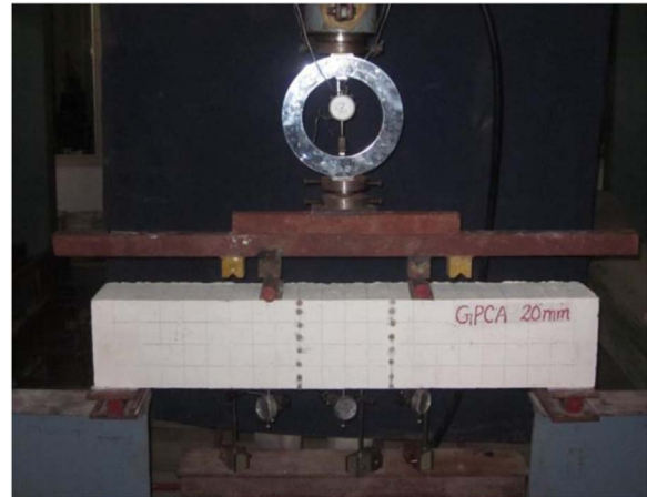
Fig. 4. Experimental set up for loading of GP concrete beam.
