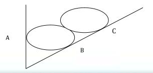
12. A string tied to a wall is made to pass over a pulley placed 2m away from it. A weight P is attached to the string such that the string stretches by 2m from the support on the wall to the location of attachment of weight. Determine the force P required to maintain 200 kg body in position for  $\theta = 30^{\circ}$ , The diameter of pulley B is negligible. (14 marks)
